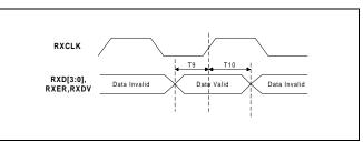
Figure 16. MII Receive Timing Parameters
